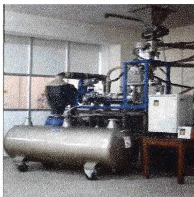
Cryogrinding facility developed at IISc.
