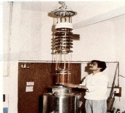
SC Magnet Developed at NPL
