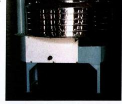
machine is recommended for roasting of powders, grains, pulses etc. It is available from 10kg to 60kg per batch. LPG is used as fuel.
